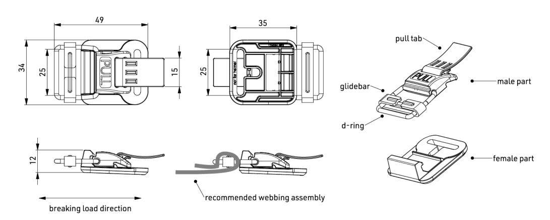
dimensions in millimeters [mm]
