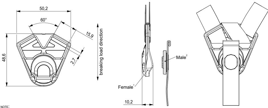
The positioning of the product on the helmet may vary depending on the size and construction, especially in the case of children's helmets. The specific application and suitability test must be carried out by the helmet manufacturer.
